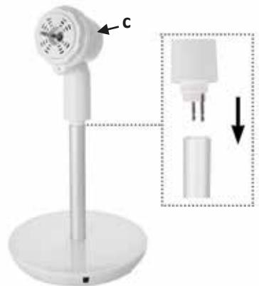
3. Attach the fan head onto the motor unit.
